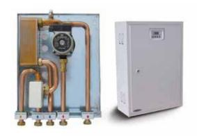
Consisting of a circulation pump, a 30 kW plate heat exchanger, a three-way diverter valve, a one-way valve and an electronic control unit. DHW storage tank separation and management kit. It makes it possible to combine a pellet or wood stove with a pre-existing system such as a gas boiler with radiators, while separating the primary circuit from the secondary one and managing a storage tank for the production of instant DHW.
